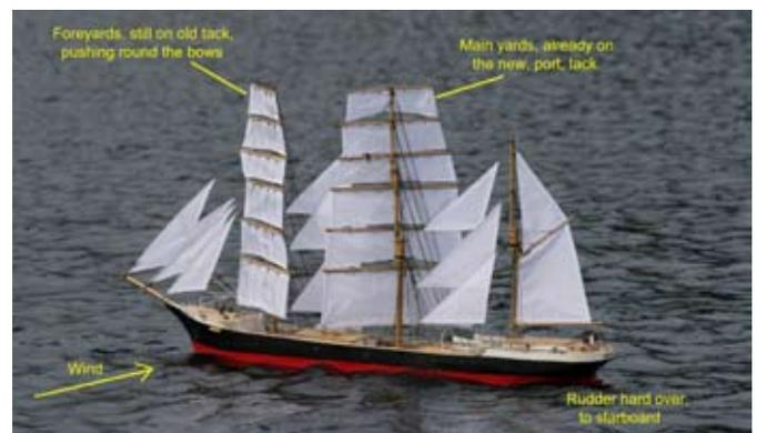
**The barque, going about from the starboard to the port tack. The main mast yards are on the new tack, and those on the fore mast are pushing round the bows, before they too are put on the new tack. Rudder to starboard gives the clue as to the direction of the turn**
